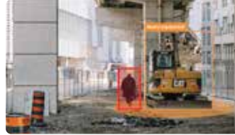
Heavy equipment approach Rapid warning when safety distance is violated
