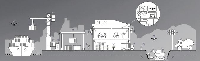
Microamp 5G mmWave covers all the interior facilities and the most crucial external areas such as loading docs and storage grounds, where CellBox Air devices are in fixed positions. For ad-hoc network deployment, mobile hotspots on vehicles are used.
