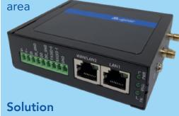
M.gear 4G LTE MII411 IoT Router and IoT Management with WAN/ LAN2 port, LAN1 port and integrated Wi-Fi, and IoT management features for device monitoring, real-time alarms and network reporting.
