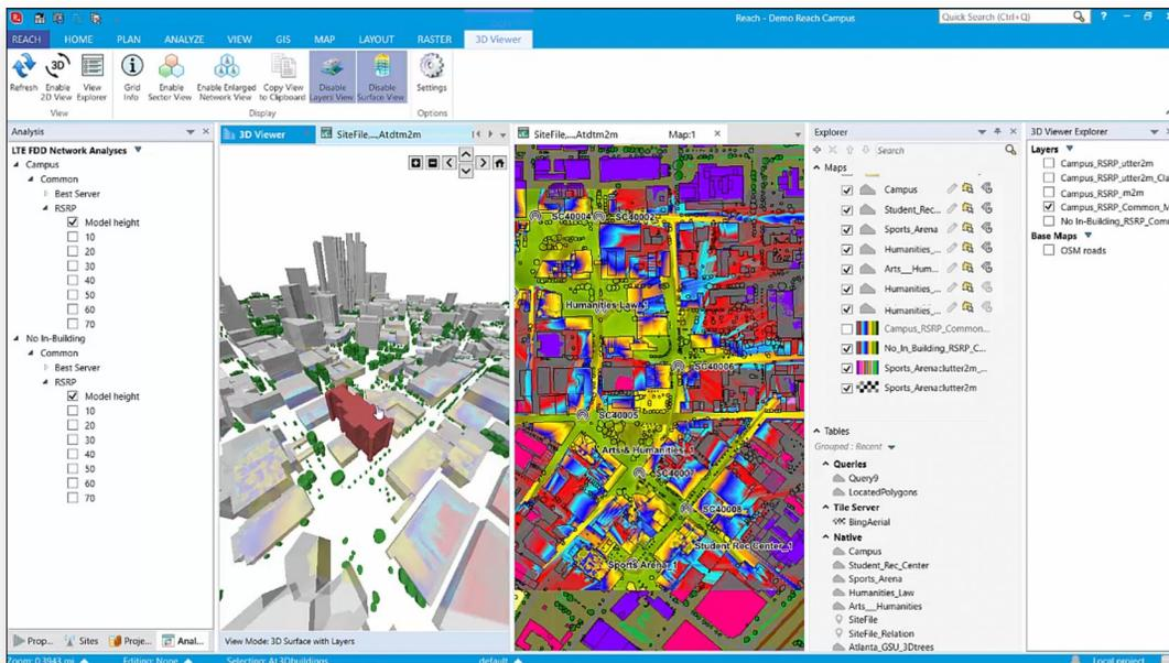
iBwave Reach's side by side windows showing the 3D building view on the left side including the in-building network data imported from iBwave Design, and on the right side showing the final result of macro penetration inside buildings and the various in-building networks' impact on the macro signal.
