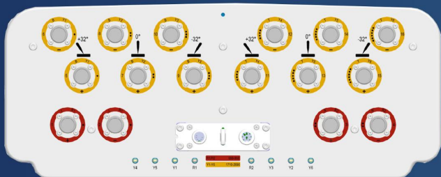
16 Ports Hybrid Multibeam Antenna U23L2PX311.510P-2C 2×698-960/2×3×1710-2690MHz 65°/2×23° 2700×498×197mm
