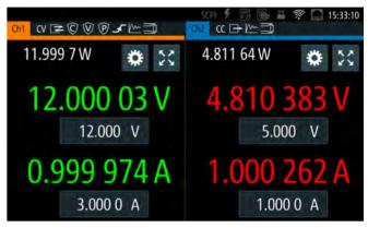
R&S\*NGM200 6 ½ digit resolution in V/I metering: With a resolution of up to 6 ½ digits when measuring voltage, current and power, the R&S\*NGM200 power supplies are perfect for characterizing devices that have low power consumption in standby mode and high current in full load operation. They are integrated into the R&S\*CMX500 with the R&S\*CMX-KM110 battery life measurement option.
