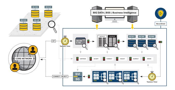
Connected directly to the operators STP's MavenShield receives CAMEL IDP triggers, and based upon the INAP IDP message content it either accepts or rejects calls.
