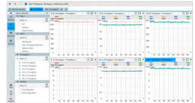
5G throughput measurements over multiple layers.
