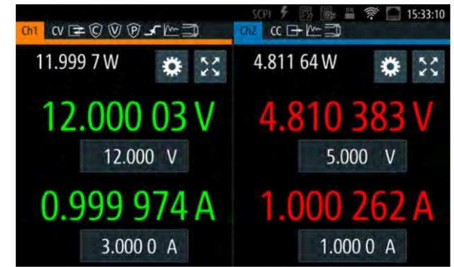
R&S®NGM200 6½ digit resolution in V/I metering: With a resolution of up to 6½ digits when measuring voltage, current and power, the R&S®NGM200 power supplies are perfect for characterizing devices that have low power consumption in standby mode and high current in full load operation. They are integrated into the R&S®CMX500 with the R&S®CMX-KM110 battery life measurement option.
