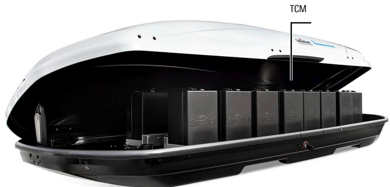
Vehicle roof box (VRB) hosting test device containment modules (TCM)
