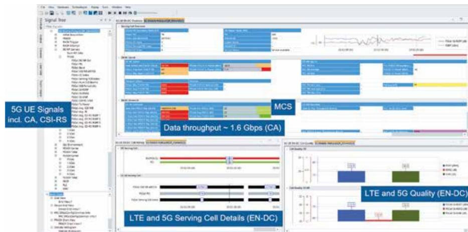
R&S®ROMES4 drive test software supports the connection of 5G NR routers, precommercial and commercial smartphones and network scanners. Scanners are passive devices for monitoring cell and beam environment of multiple networks. Adding 5G UEs enables monitoring of 5G NR device-network interaction and UE specific channels and data streams, including special features and metrics such as 5G carrier aggregation, dynamic MCS, access procedures, 5G mobility and application performance.
