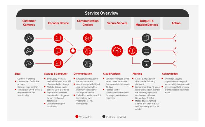
Unlike China Telecom, Vodafone offers encoder devices with storage and video analysis capabilities that can be connected to customers' networks. These devices then upload alerts and related videos to a cloud platform via cellular networks or fixed lines, providing end customers with remote monitoring capabilities.
