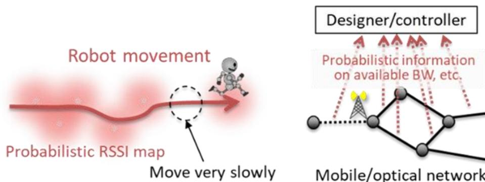
Figure 11 Use Case Examples of Network Digital Twin for Radio Communication Environment
