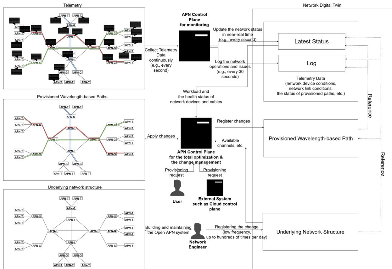
Figure 3 Network Digital Twin for the CPS Network Infrastructure Management Use Cases
