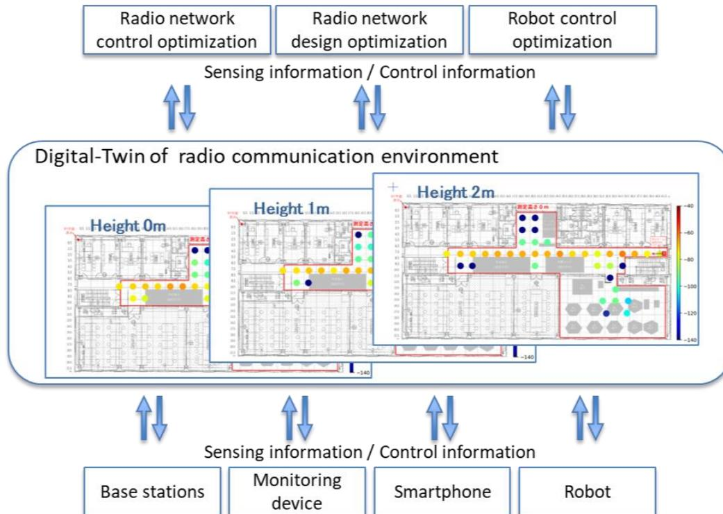
Figure 10 Network Digital Twin for Radio Communication Environment
