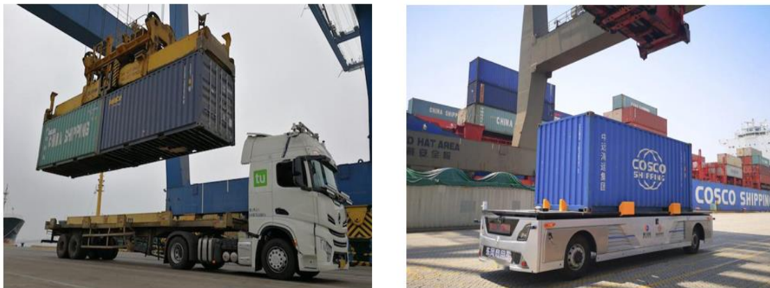
Figure 8-10 Autonomous Drive Container Trucks and AGVs
