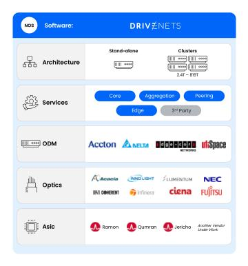
True diversity on all fronts – mixing and matching of disaggregated NOS, ASIC, ODM, optics and service components
