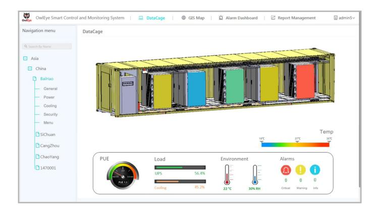
DataCage is the product developed to address this need in the market. Other than typical mobile data centre, DataCage offers mixed IT (information technology) and CT (communication technology) power and energy infrastructure in a prefabricated ISO container allowing immediate installation of server and telecom equipment to shorten the deployment and commissioning time. DataCage is designed to operate in various terrains as well as harshest environments.
